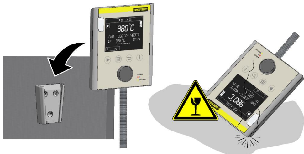
Fig. 18: Place the controller in the holder on the furnace (similar to the picture)
