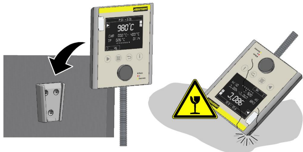
Fig. 27: Place the controller in the holder on the furnace (similar to the picture)
